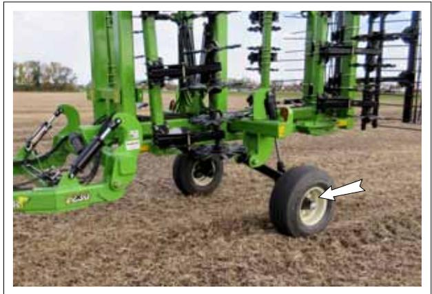
**Fig. 45 WHEEL BEARINGS (Typical)**
