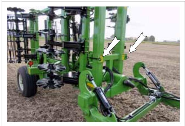
Fig. 37 TRANSPORT LOCK PINS
