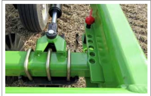
Fig. 34 ANCHOR PINS
